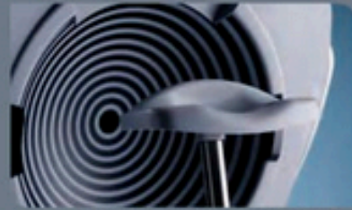
Placido disk - Measurement of corneal curvature radius
